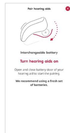
Figure 12: Instruction Interchangeable battery
